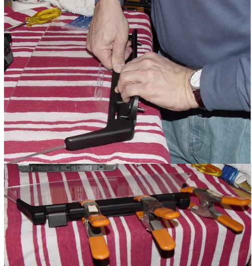
12. Let the glued and clamped assembly cure for at least 24 hours, then remount the screen to the car, following the first part of these directions in reverse. When you remount the screen mechanism on the car, apply the anti-vibration bumpers supplied with the screen, following the separate instructions included.
