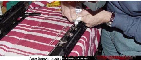
get any of these glues on the screen. Wipe them off immediately if you do. This gluing is critical to the integrity and durability of the of the mechanism and screen, so be sure to do the job right to ensure that the mechanism is solidly glued together.
