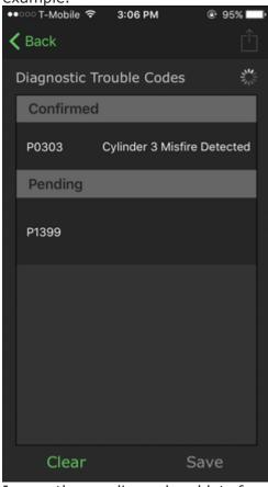
Ignore the pending cel and lets focus on the P0303 which is cylinder 3 misfiring. Move the coil to another cylinder and then clear the code. I moved it to cylinder 2, cleared the codes, start the car, let it run and boom.
