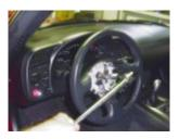
Now use the steering wheel puller you've rented (or bought) to remove the wheel. There are two holes just outside of the hub bolt/nut; use these to mount the puller, with the center bolt of the puller pressing against the hub nut/bolt:
