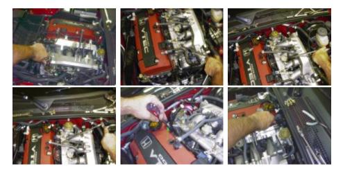
Note that you have to remove a cable clip to get to the last nut on the top. I also found that I could only get to it with a wrench, not with a socket.
