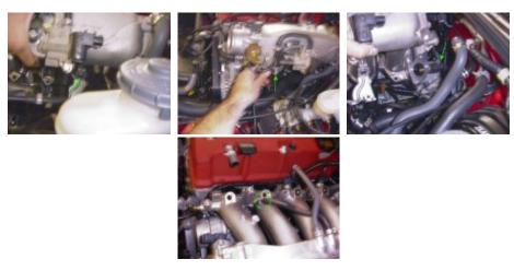
Last, we have the throttle cable. The throttle cable is on the driver's side and is secured by a 12mm locknut:
