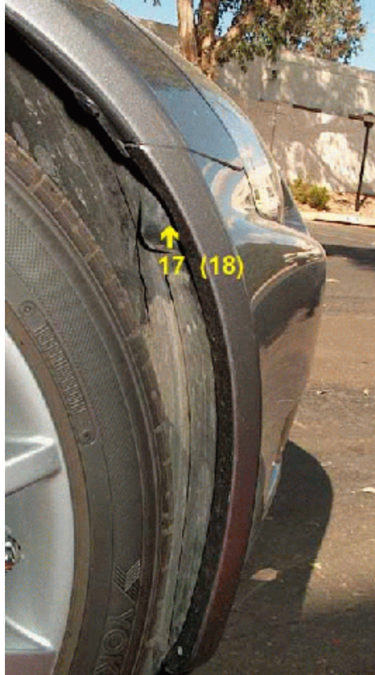
Figure 4 Wheel well screw location
