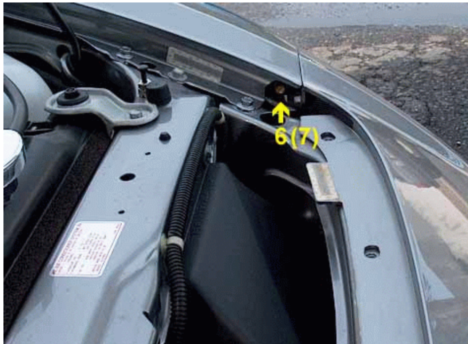
Figure 2 Fender Bolt location
