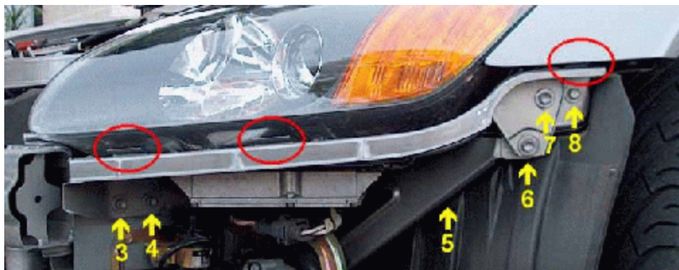
Figure 8 Corner upper beam bolt locations
