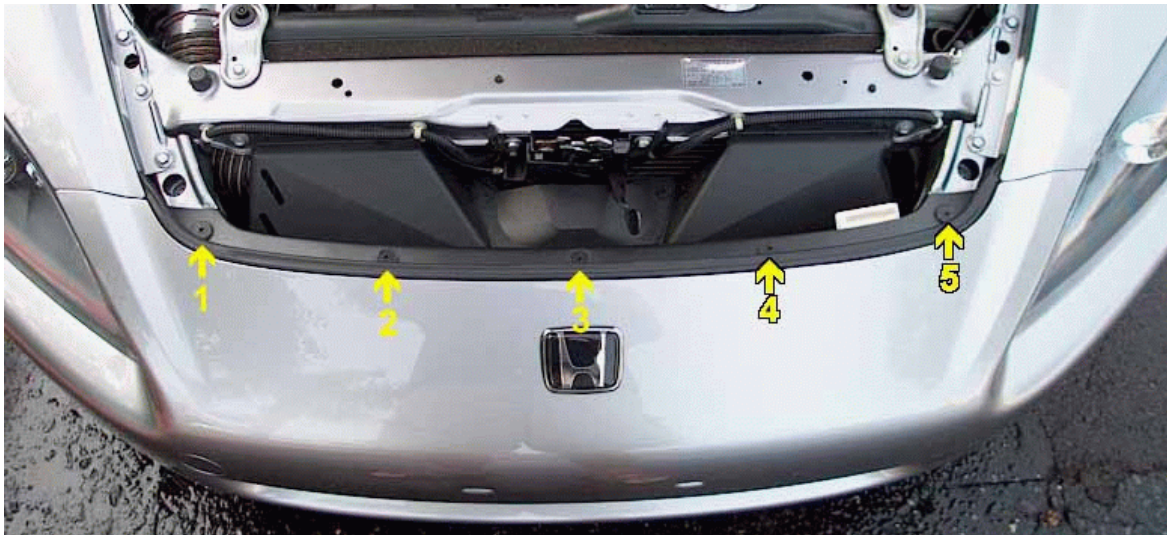
Figure 1 front bumper upper stiffener bolt locations (1-5)
