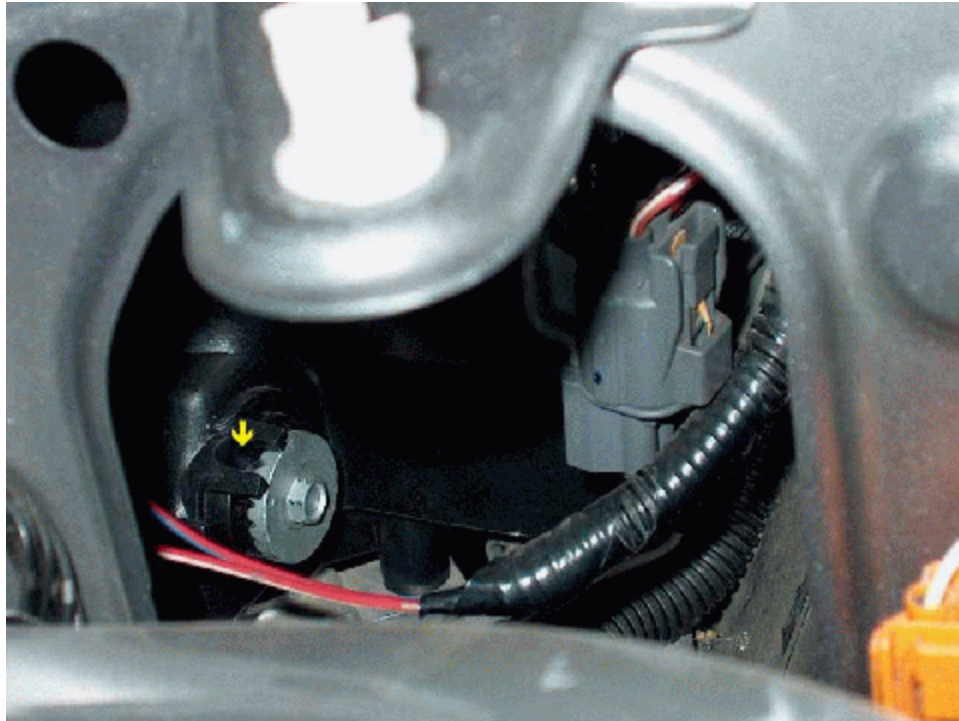
Figure 11 Headlight vertical adjuster location.
