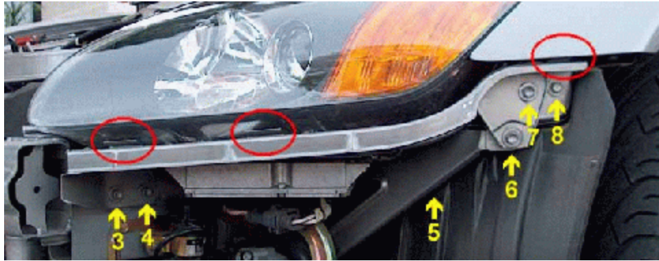
Figure 5 Four bumper hooks under the headlights locations (circled in red)
