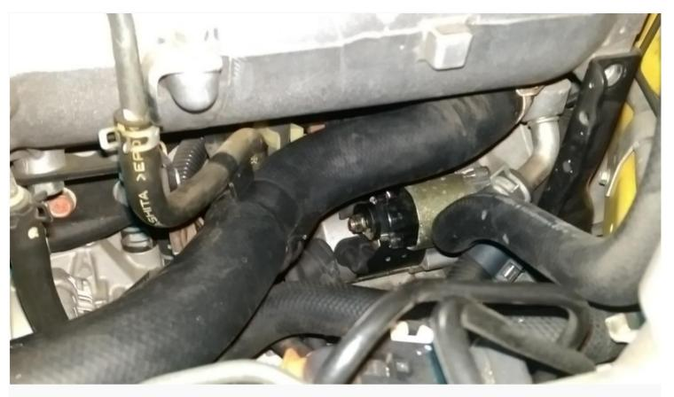
6) Unplugged the knock sensor (green plug in pic), the knock sensor is plastic and brittle. Don't break it. Seriously, its easy to do. Move that section of wiring harness out of the way to get a better view of starter.
