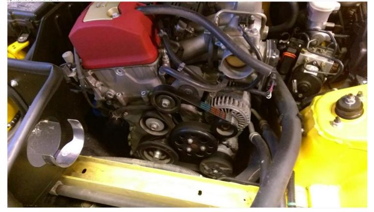
3) Remove Accessory Belt, take tension off with wrench and take belt off the alternator pulley.
