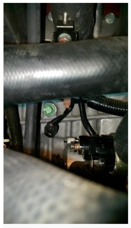
7) Remove the top bolt of the starter, you will need a long extension and a 14mm swivel socket helps.
