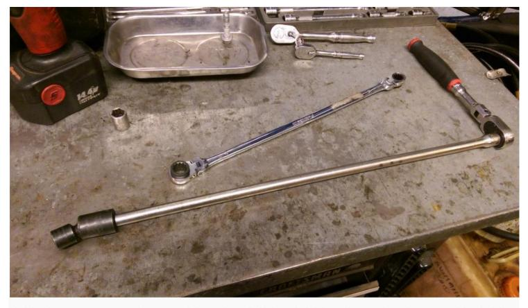
I find that the easiest way to get on the top starter bolt is to shine a flashlight on the bolt from in between the intake runners and then feed the swivel socket in from the front towards the light. Remember don't break the knock sensor!
