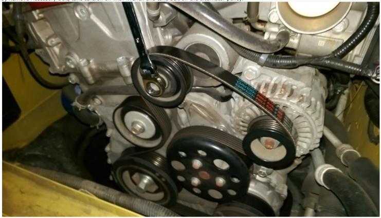
4) Remove top bolt of Alternator, losen lower bolt and rotate the alternator to the right.
