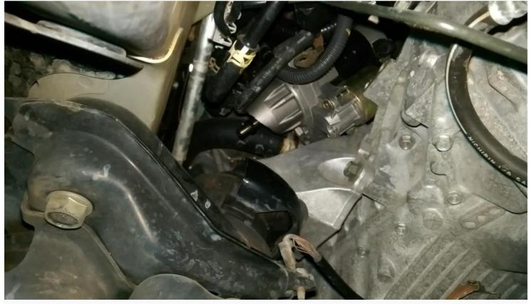
12) Twist and rotate starter to get it out. Takes a little time and finesse. Don't forget about that knock sensor.
