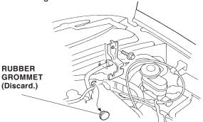
13. Get the hood switch harness. Using a utility knife, cut off and remove the marked area of the rubber grommet. Be careful not to damage the hood switch harness.
