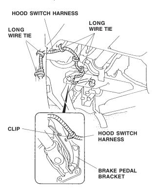
23. Secure the hood switch harness to the vehicle harness with five long wire ties in the areas shown.
