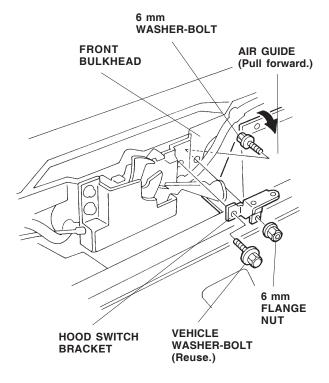
Remove the tape and the two screws that fasten the hood switch to the existing switch bracket, then remove and discard the existing bracket. Save the screws; they will be reused.
