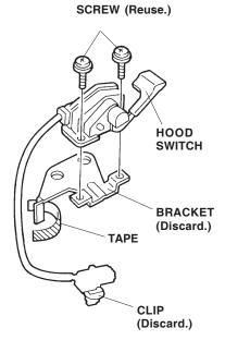
7. Remove and discard the clip from the hood switch connector.
