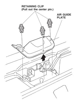
4. Remove the two retaining clips from the left (driver's) side of the air guide.
