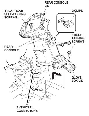
24. Using a felt-tip pen, mark the indicated positions on the rear console box.
