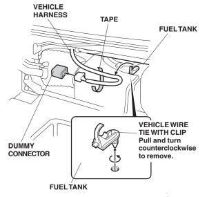
Route the adapter unit harness as shown and connect the adapter unit harness 14-pin connector to the vehicle harness 14-pin connector.
