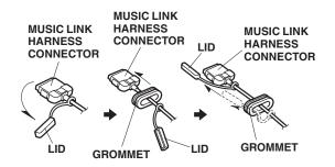
33. Route the Music Link harness connector through the hole made in the step 27, then route the lid through the hole as shown.
