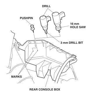
26. While wearing an eye protection, drill 3 mm holes at the two locations marked in step 25, and then enlarge the holes with 16 mm hole saw.
