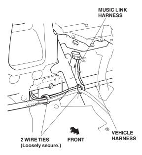
32. Remove the Music Link harness connector lid, and put the Music Link harness connector through the grommet, then put the lid through the grommet.
