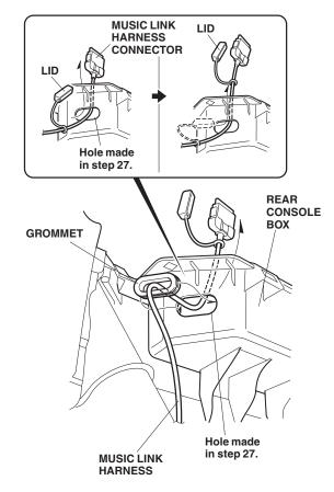
34. Reinstall the Music Link harness connector lid. Install the grommet in the rear console box.
