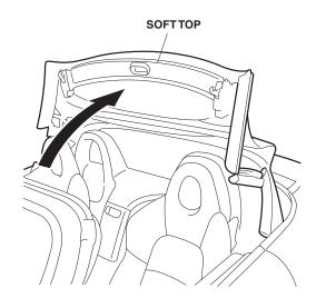
6. Raise the rear glass and pull out the rear tray. Do not damage the heater wires of the rear glass. Remove the rear tray while moving the soft top and the rear glass.
