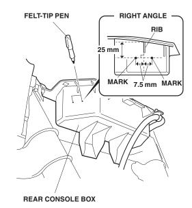
25. Using a pushpin, mark the rear console box at two locations marked in step 24.
