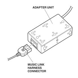
30. Route the adapter unit harness. Secure the adapter unit with a 5 x 8 mm bolt and a 5 mm plain washer to the vehicle frame. Secure with the 5 x 8 mm bolt while holding the 5 mm plain washer with your finger.
