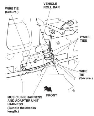
41. Secure two wire ties loosely secured in step 31.
