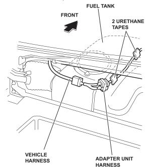
40. Bundle the excess Music Link harness and the adapter unit harness with two wire ties and secure it to the vehicle roll bar. Secure the wire tie at the tape attached in step 28.
