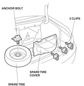
8. Remove the anchor bolt and remove the spare tire. Go to step 14.
