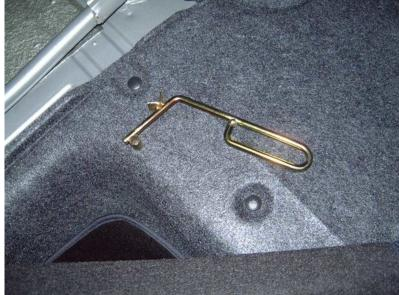
Use the trunk spring remover to take off the trunk spring. Its not that hard to remove the trunk spring with the right tool.
