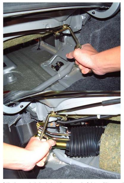
Putting the new spring back on is almost the exact opposite of what you did to remove them. I rest the trunklit on my back when removing and installing the spring.
