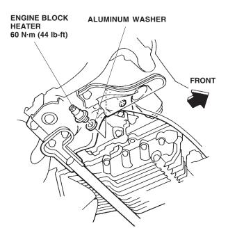
Attach the two wire ties with clip to the heater harness in the areas shown.
