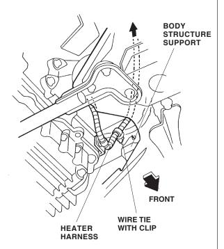
10. Continue routing the heater harness along the vehicle harness as shown.
