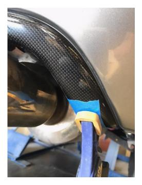
4. It is recommended to use the pre-drilled holes on each end of the cover as a template and drill the holes for the securing hardware.
