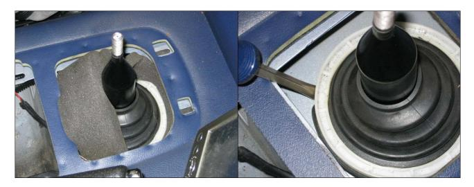
5. Pull the rubber cover up and twist it around to expose the (3) 10mm bolts
