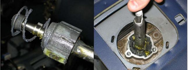
10. Place the retaining collar over the shifter and line up the bolt holes. Notice the orientation of the indentation on the inner surface of the collar points toward 6<sup>th</sup> gear.
