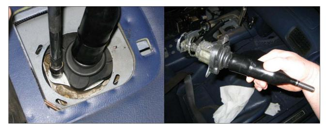
8. Pull the spring off the end of the stock shifter and install it onto the short shifter.
