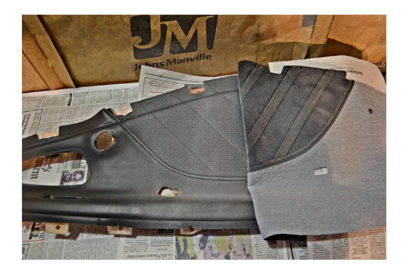
Next move on to the last section. Make sure it is pressed down from the middle outwards to ensure there is no material that is not glued down. If the outside edges touch first it will be difficult for the middle to be pressed together.
