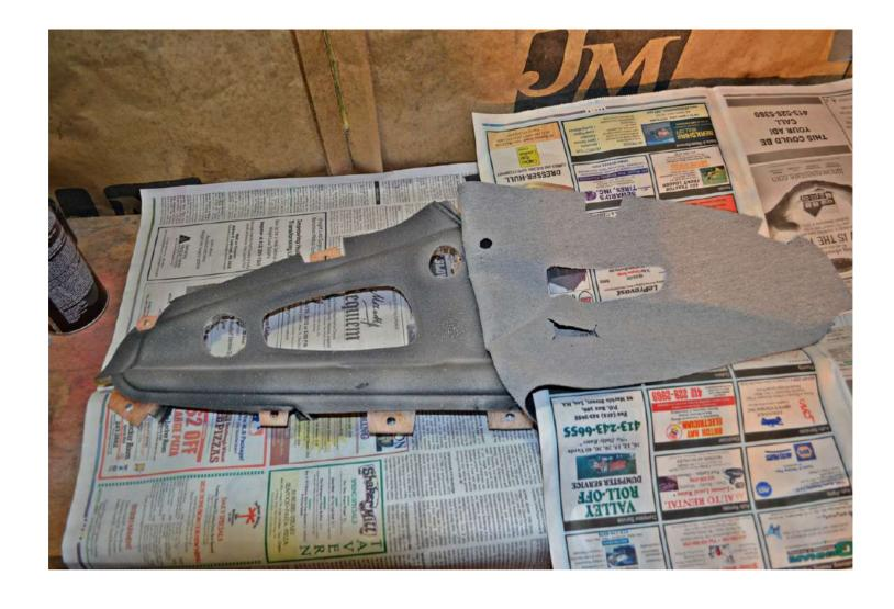
Now it should be entirely covered. The holes for the door handle will need to have slits cut so you can re install the door handle.
