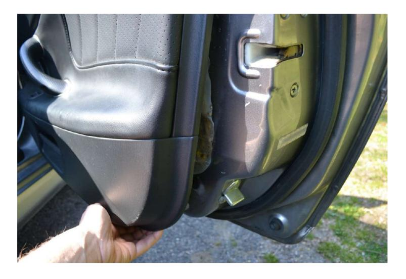
There is a plug on the backside for the window switch that will need to be removed and if you have tweeters installed those will have to be disconnected as well.
