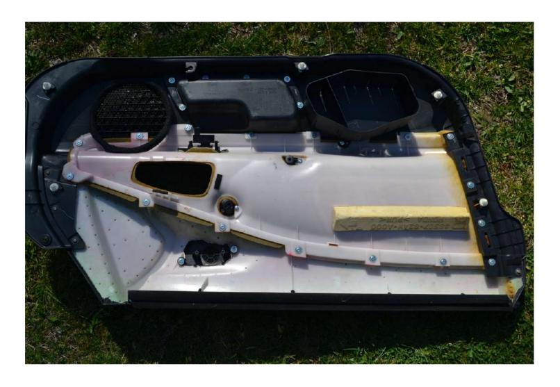
First remove the door handle. There are 2 screws holding it in place from the backside. As you can see there are lots of screws holding the door insert onto the whole interior door panel. All (16) must be removed.
