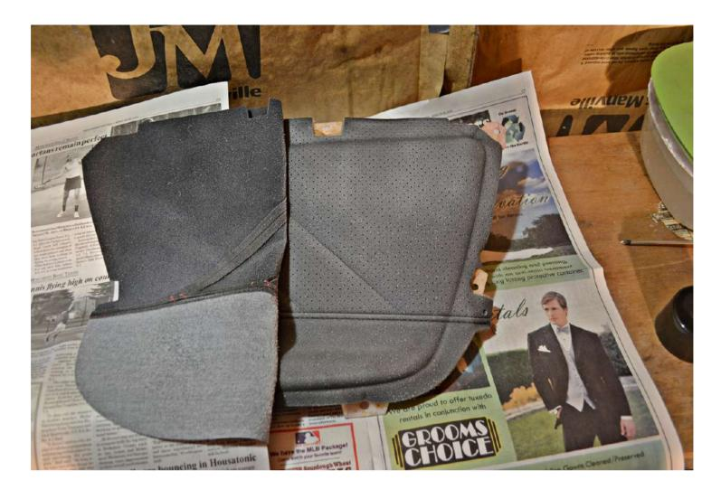
Now carefully press the door insert cover over the door insert. Make sure there are no creases and it is covering al the material that will be showing. Make sure it is tight in all spots.
