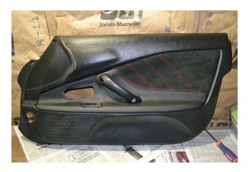
You are now DONE with the door insert cover installation. Now just need to reverse the steps to install the door panel back into the car. Make sure you remember to plug the window switch plug back in.
