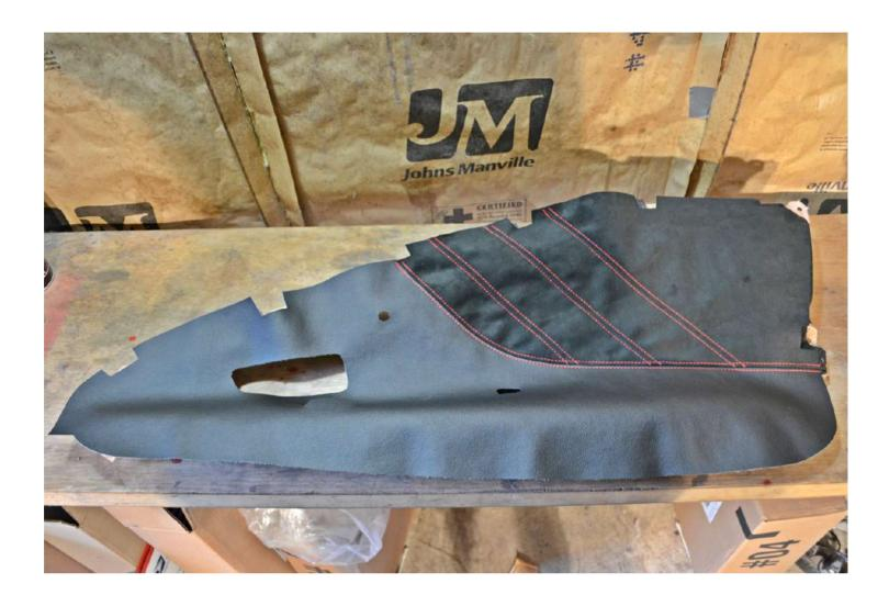
Once you have determined the best spot to overlay the door insert, have someone hold it in place. I found it works best to start at the back end and do it in 1/3 sections.
