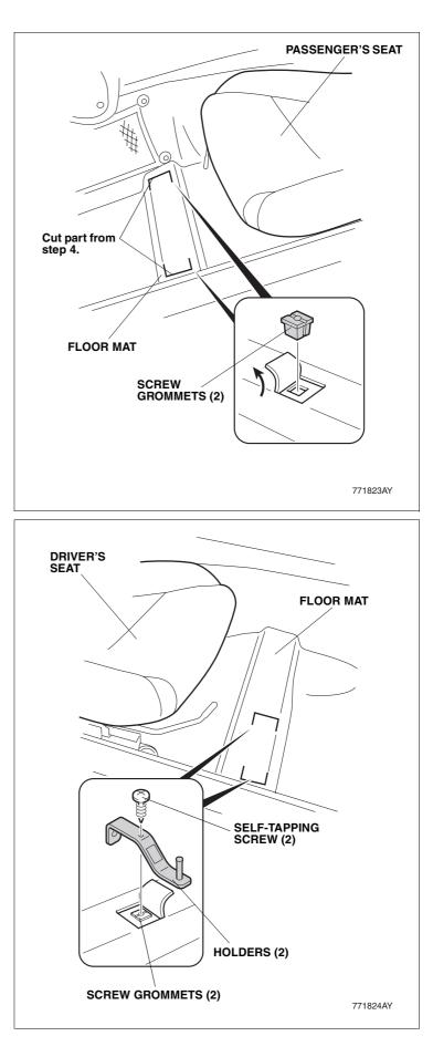
7. Install two holders to two screw grommets on the driver's seat side as shown (two self-tapping screws).
