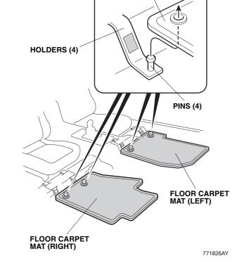
11. Install the cover mat (right) onto the driver's seat side holders (two magic fastener and two hooks).
