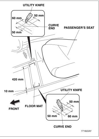
6. Pell off the part of the floor mat cut from step 4 and install a screw grommet into the square hole.
