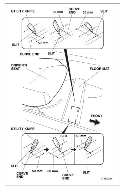
3. Peel off the part of the floor mat cut from step 2 and install a screw grommet into the square hole.
