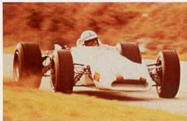
Richie Ginther drove this car to Honda's first Grand Prix win. His victory took place at the 1965 Mexican GP. The car is powered by a 1.5 liter V-12, mounted laterally in the chassis.
