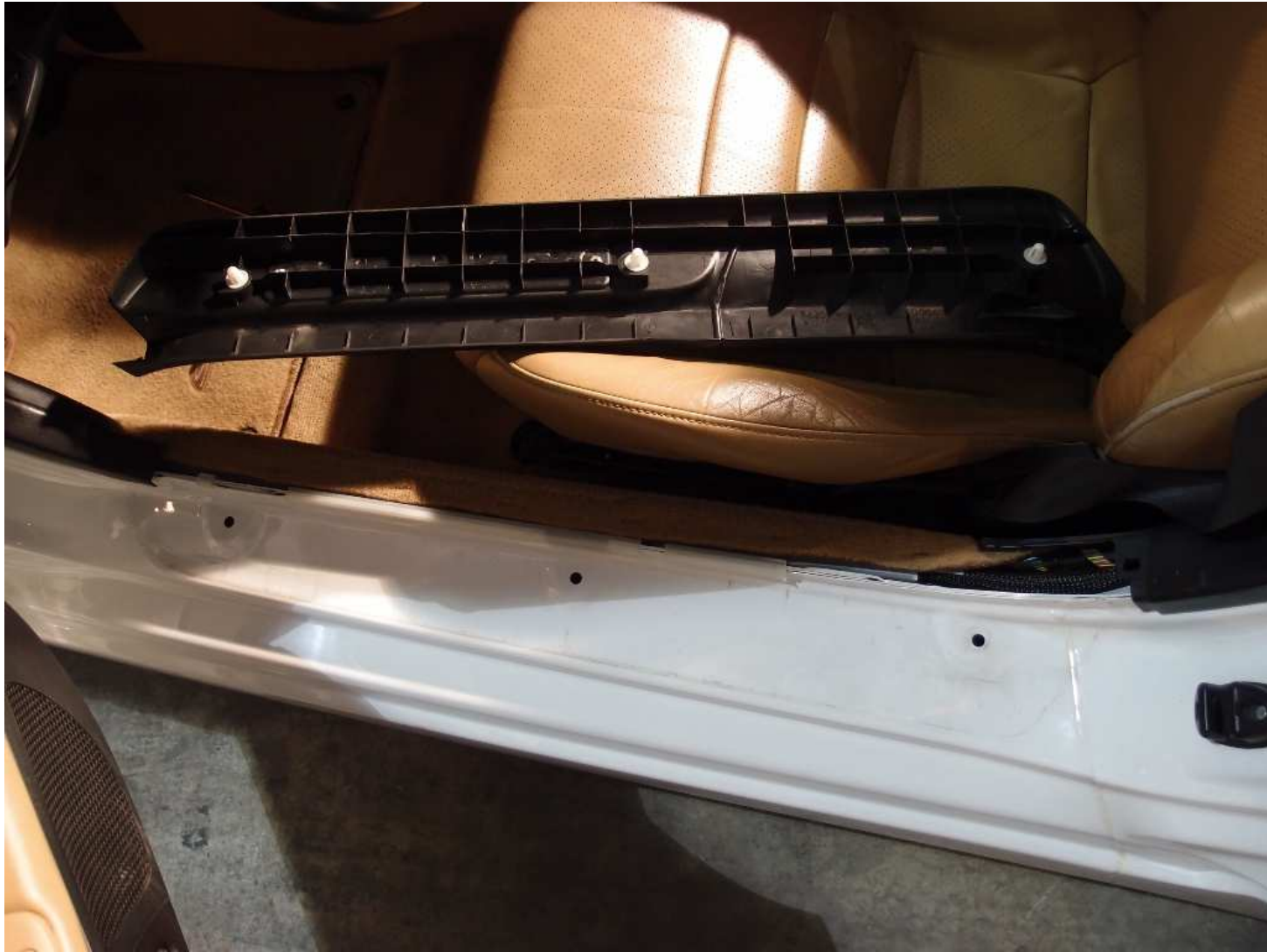
02. JPG Left door sill cover removed.
