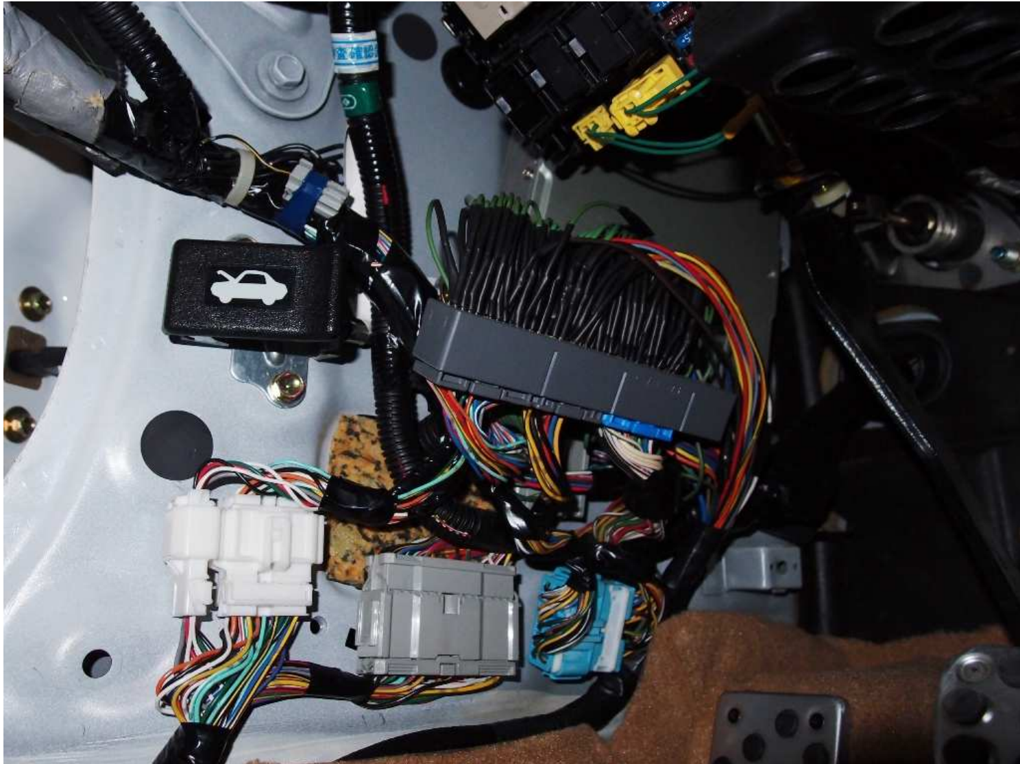
07.JPG This shows the PNP harness installed.
