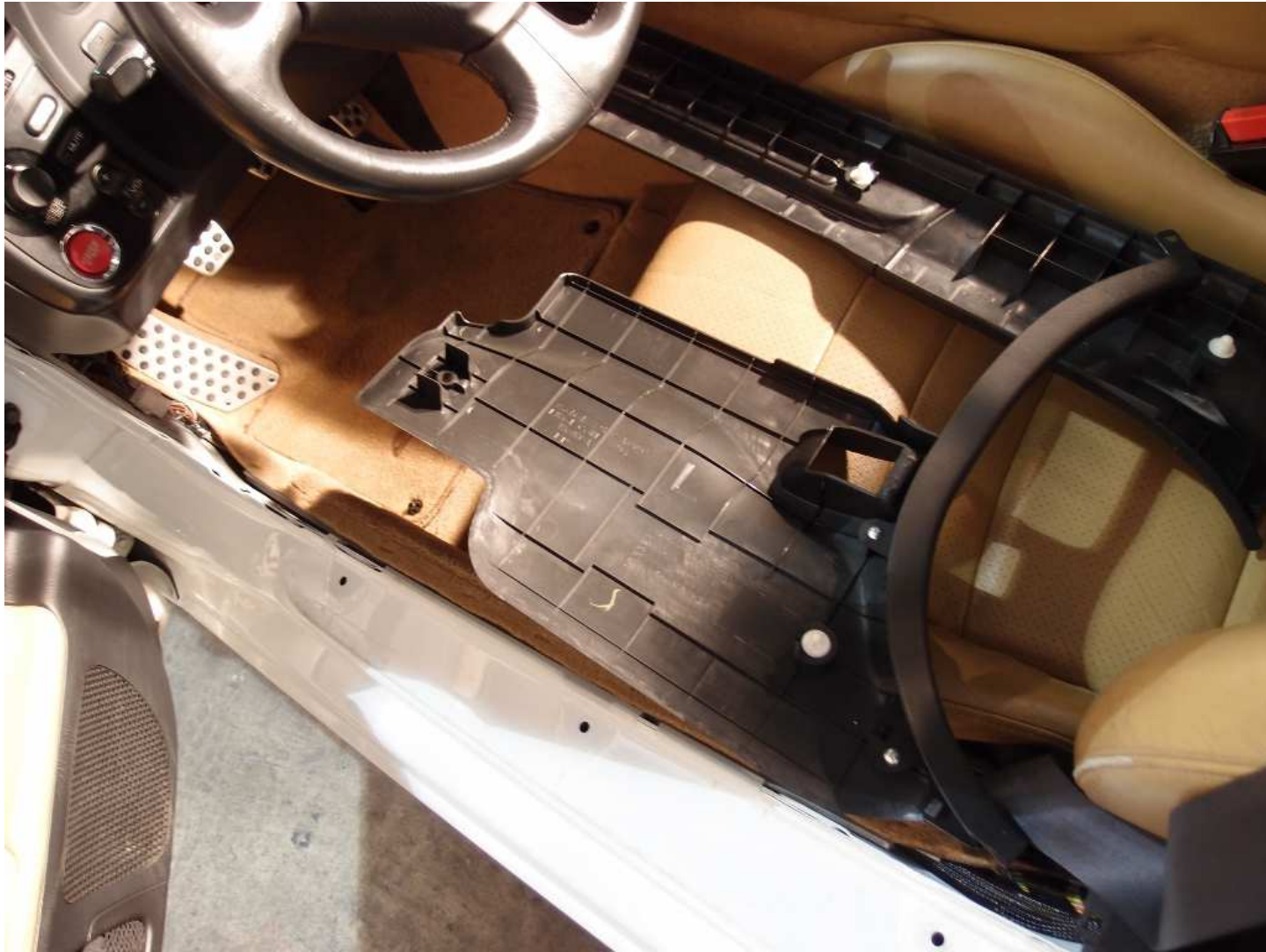
05.JPG Panels removed. Set aside.
