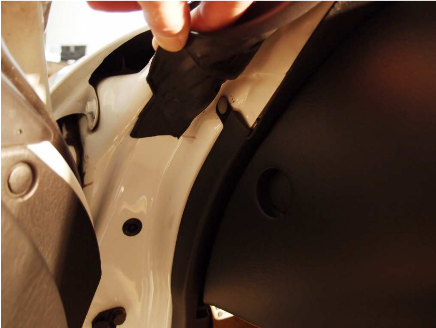
04.JPG Shows the location of clip 17 under the weather-stripping
