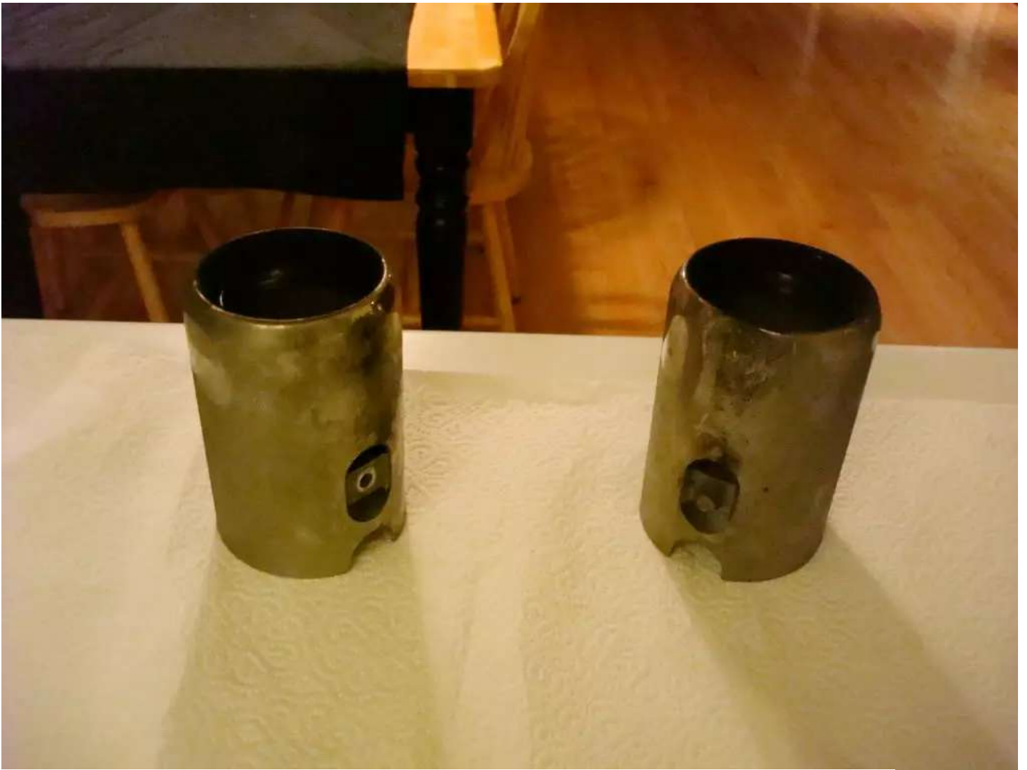
The exhaust tips are purely cosmetic on the OEM muffler so they come off with a single bolt (10mm)
